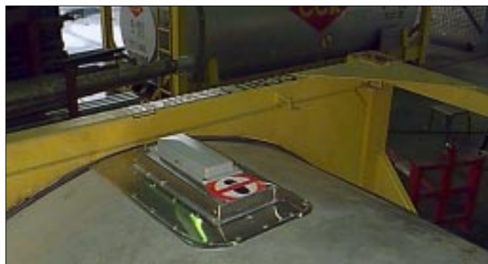
An AGT transmitter installed on a CCR tank container
